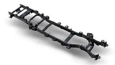
Heavy commercial vehicles such as trucks and buses mainly use the ladder frame structure. Some light commercial vehicles like pickup trucks also use the ladder frame.
