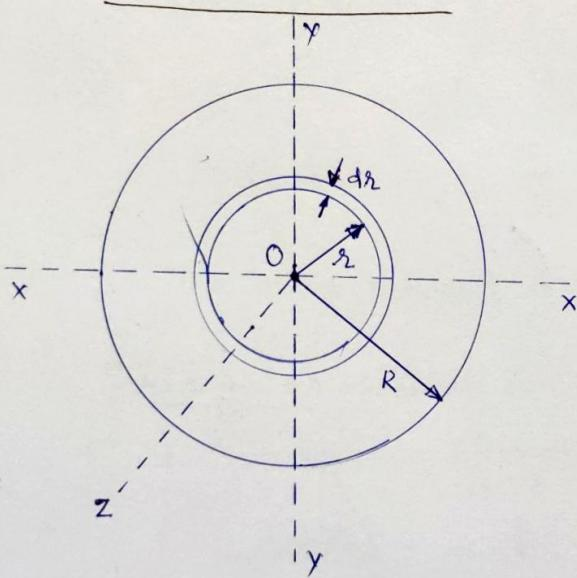
Consider two mutually perpendicular axes  $x-x$  and  $y-y$  passing through the center of circle of radius  $R$ .
