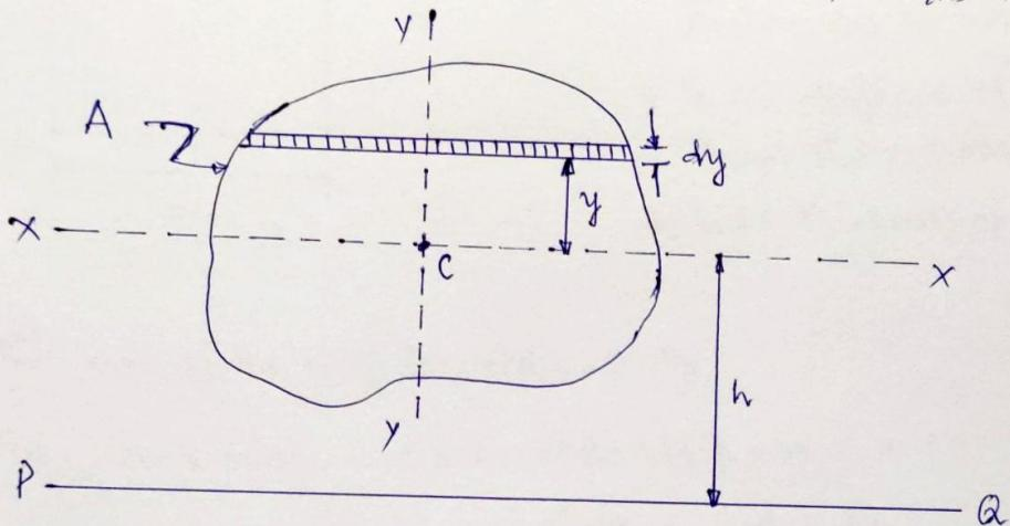
Proof: Consider an elementary strip of area  $dA$  at a distance of  $y$  from the centroidal axis  $x-x$  which is parallel to reference axis  $PQ$ , so that the distance of the strip from reference axis  $PQ$  is  $(h+y)$ .
