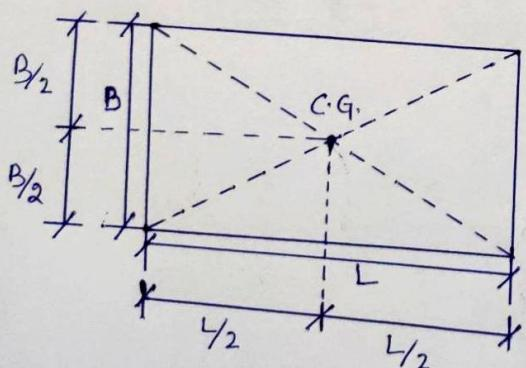
Here, the centroid is at that point where its diagonals meet each other. It is also a middle point of the length as well as the breadth of the rectangle.
