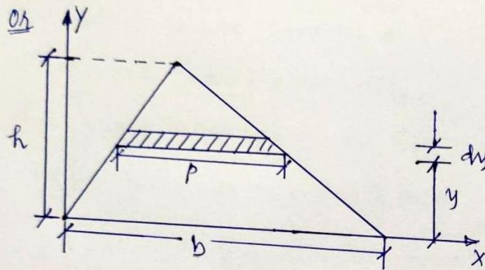
At a distance  $y$  from  $x$ -axis, a differential element is chosen of thickness  $dy$ . from the concept of similar triangles,
