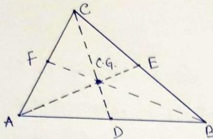
Here, the centroid is that point where the three medians of the triangle meet as shown in fig.
