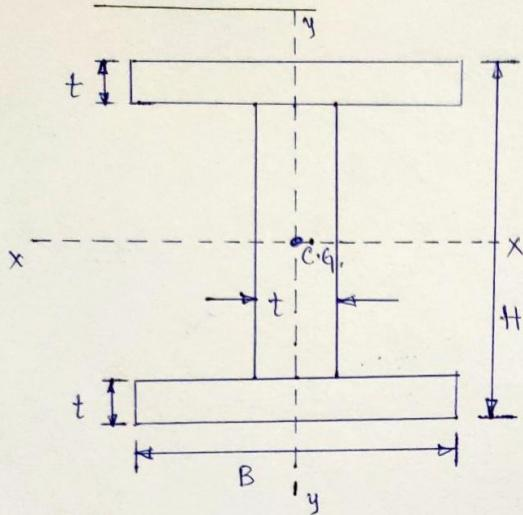
The I-section can be considered as a hollow rectangular section, where  $B = B_t$ ,  $D = H - 2t$  and
